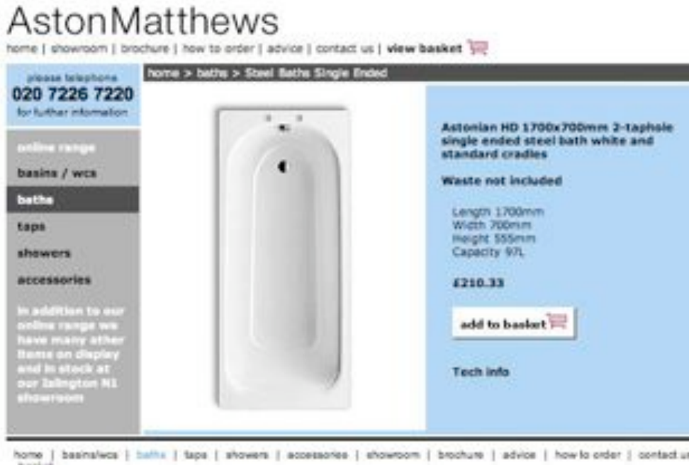
Figure 9. This 97 litre bath sounds very economical but it would be 167 litres filled to the overflow.
