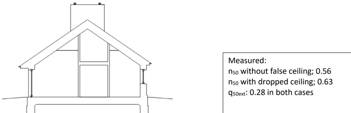
Figure 1. Example from Racecourse Estate, UK where the late addition of dropped ceilings changed the  $n_{50}$  result from pass to fail.
