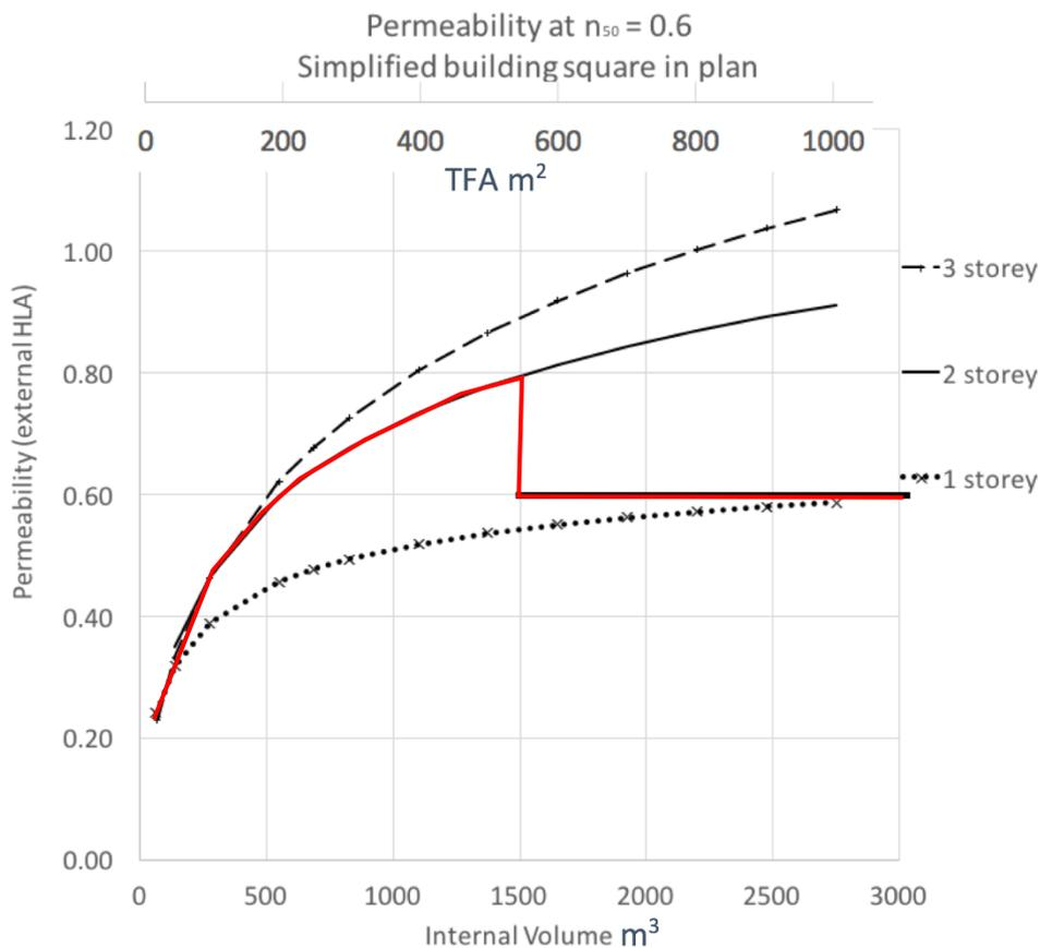
Graph 1. shows how the required permeability ( $q_{50}$ ) to meet the  $0.6 \text{ h}^{-1} n_{50}$  target varies with building size ( $25 \text{ m}^2$  to  $1000 \text{ m}^2$  TFA). The horizontal line illustrates the emerging requirement for a  $q_{50}$  of 0.6 for buildings with an internal volume greater than  $1500 \text{ m}^3$ .
