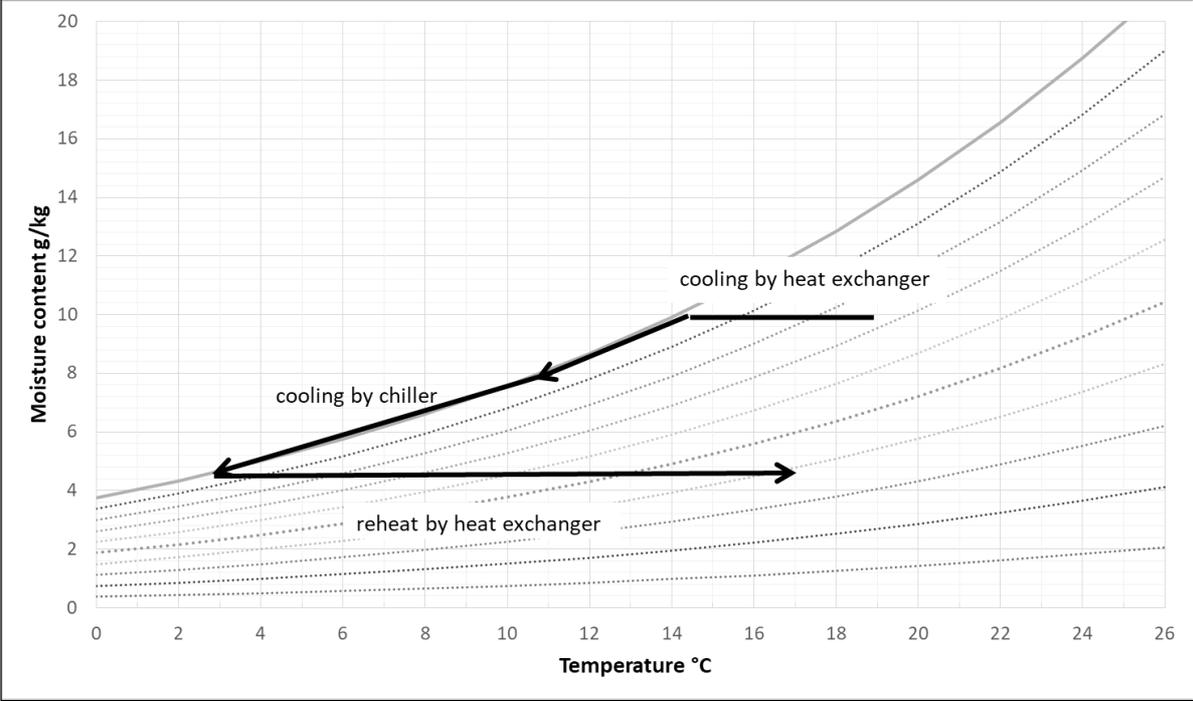
Figure 6. Psychrometric diagram of process.
