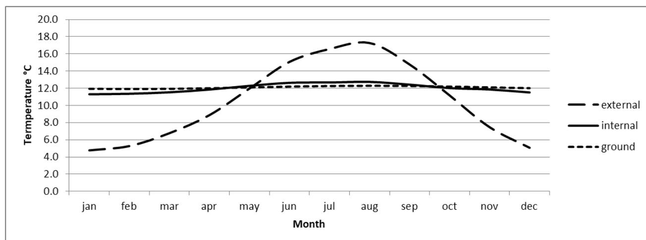
Figure 3. Modelled repository temperatures.
