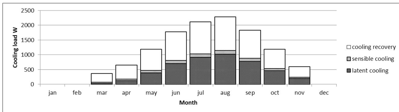
**Figure 7. Average monthly chiller load including effect of heat recovery.**
