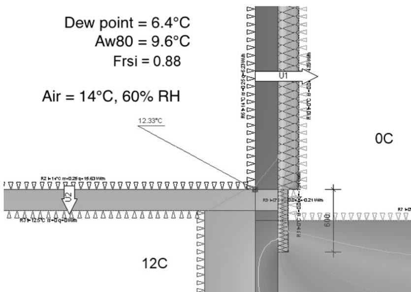
Figure 2. Ground coupled slab with edge insulation to avoid mould risk (repository temperature 12°C).
