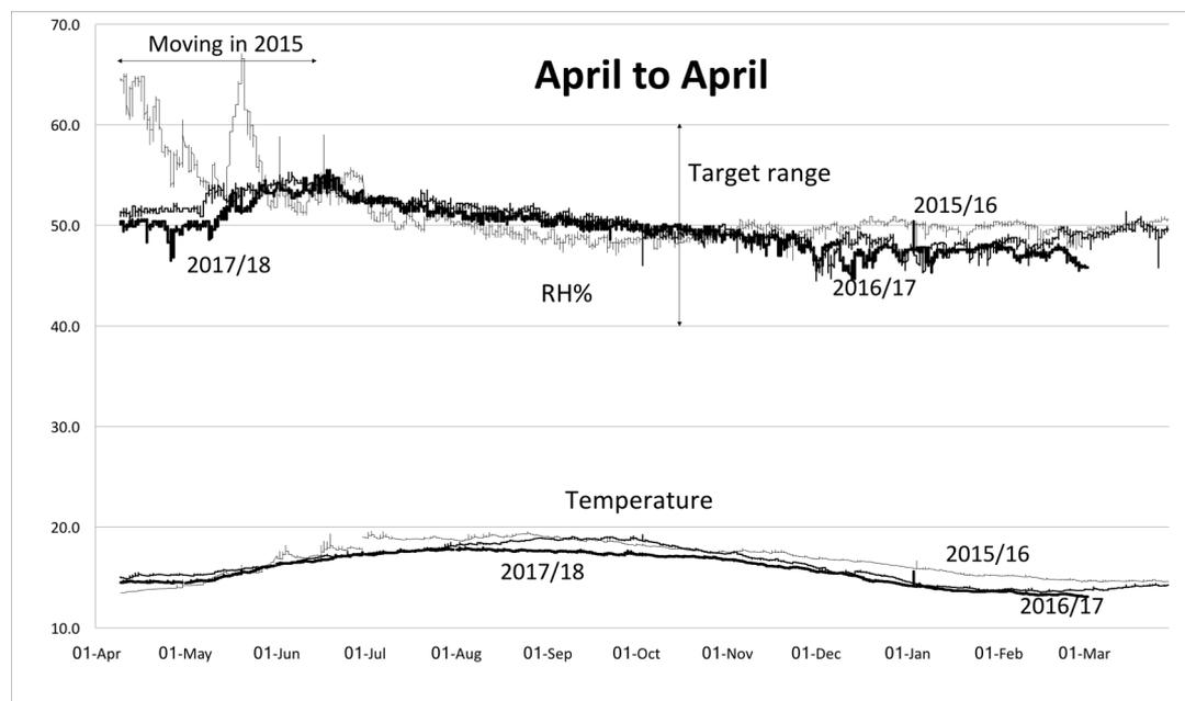
Figure 1. Temperature and RH monitoring of the middle floor of HARC since practical completion.
