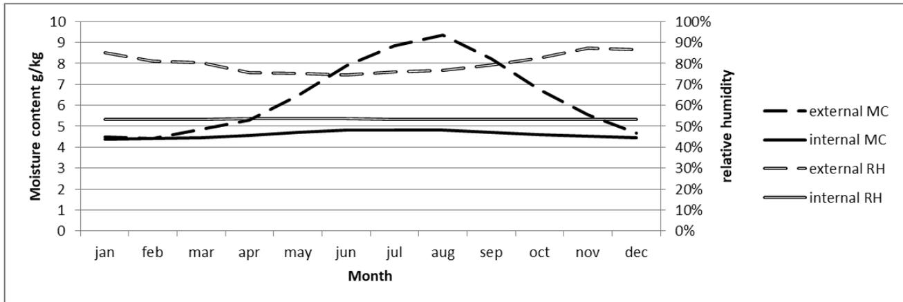
Figure 4. Modelled air absolute moisture content and relative humidity.
