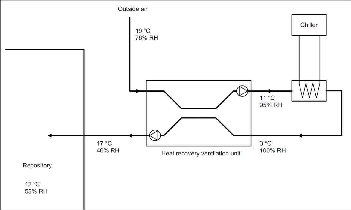
Figure 5. Supply air dehumidification with energy recovery.
