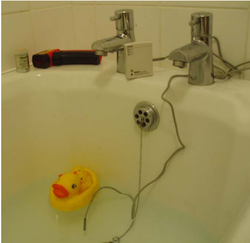
Figure 26. Space heating gains from the bath were calculated from experiments. Surface temperature (infrared thermometer) and room temperature were both measured. Bath temperature was measured (probe suspended in the water by Delyth the Duck)
