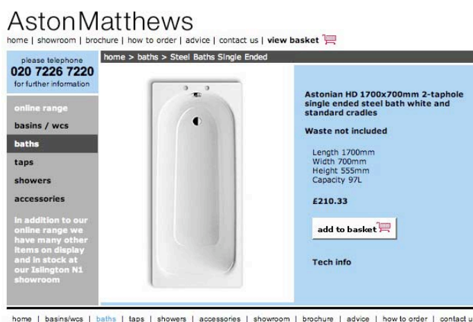
Figure 1. 97 German litres or 167 UK litres. Continental bath volumes are quoted allowing for bather displacement. This confusion is being exploited, probably in innocence.
