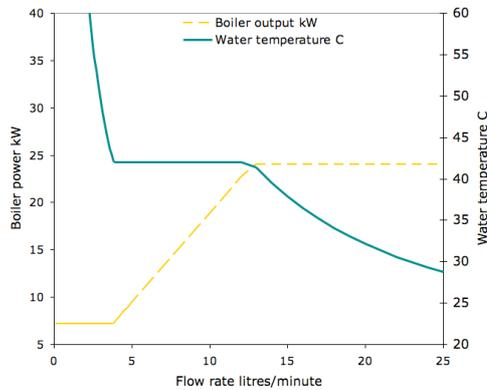
Figure 5. 24kW, modulation to 30%.
