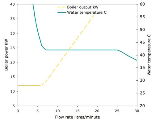
Figure 8. 48kW, modulation to 25%.
