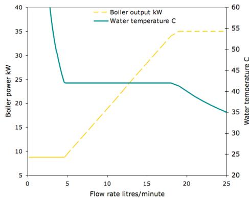
Figure 6. 35kW, modulation to 25%.
