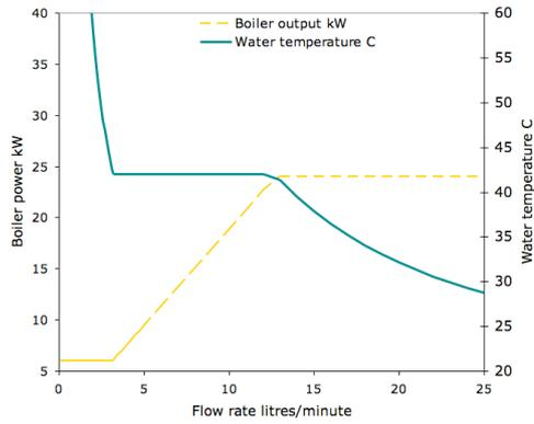
Figure 4. 24kW, modulation to 25%
