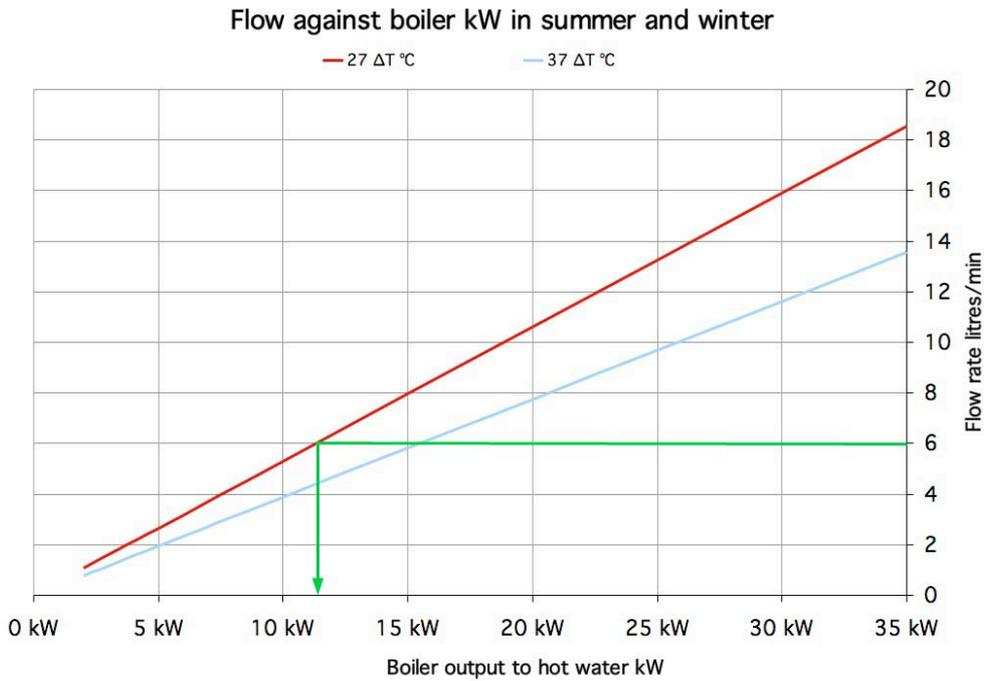
**Figure 2. Graph of flow rate against boiler output for assumed summer and winter mains water temperatures of 15 and 5 °C**
