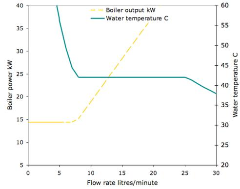
Figure 9. 48kW, modulation to 30%.
