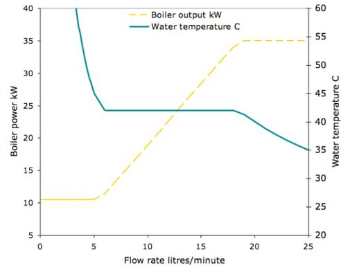
Figure 7. 35kW, modulation to 30%.
