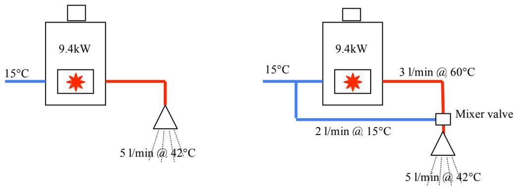
**Figure 1. Illustration showing the simplification used for the graphs and tables in this paper and the equivalent situation of boiler water mixed with cold.**
