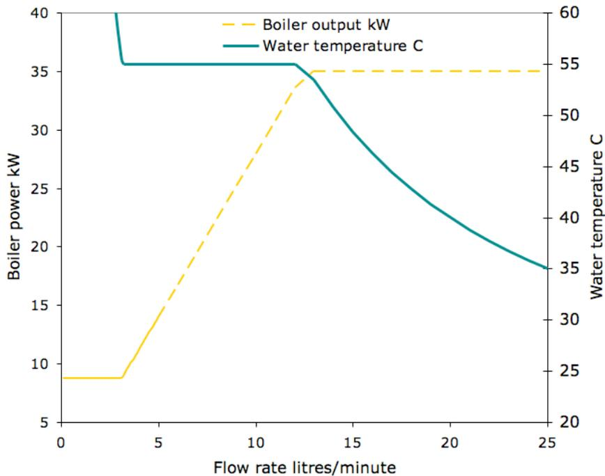
**Figure 3. Graph showing (theoretical) water temperature variation with flow rate for a 35kW boiler modulating to 25% of rated output. The hot water temperature is set to 55°C and the boiler maintains this within the modulation range. As this hot water must be mixed with cold, the final flow rate from the tap will be higher.**
