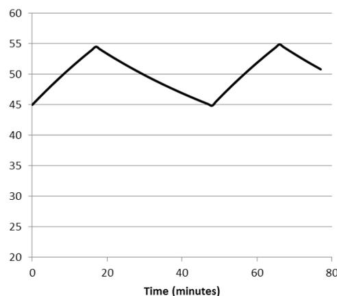
Figure 2: Calculated heating system thermal mass and temperature response with oversized radiators
