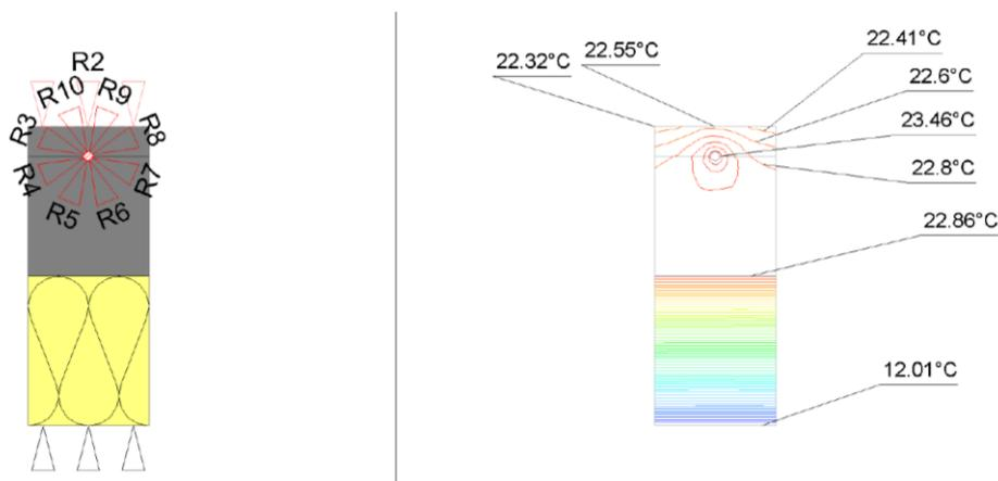
Figure 5: PSI-therm 2-D model of underfloor heating pipe in concrete slab (R2 defines room boundary condition, R3–R10 to pipe section approximated as an octagon)
