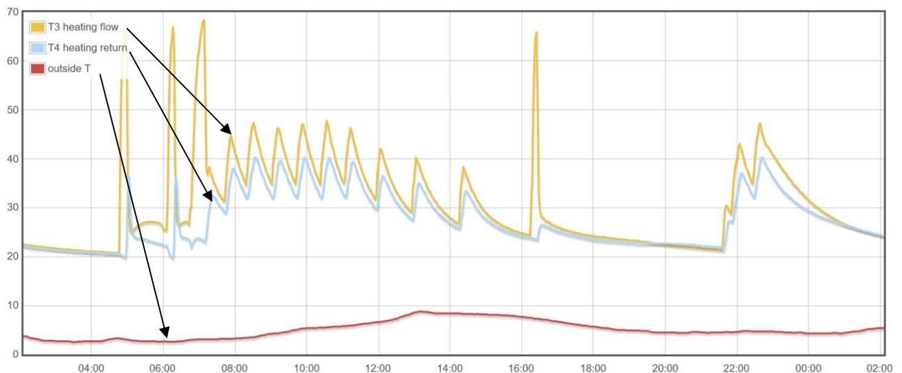
**Figure 3: Heating system flow and return temperatures during a January day**
